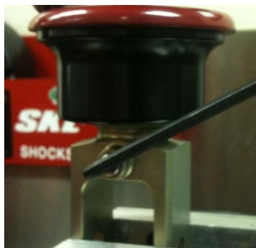
3.) 5/32" Allen Key for Compression/Rebound Adjustment
